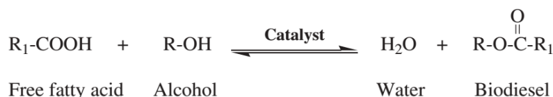
Figure 2 – Esterification of FFA into biodiesel [2]
